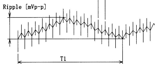
Fig. Complex Ripple Wave Form
