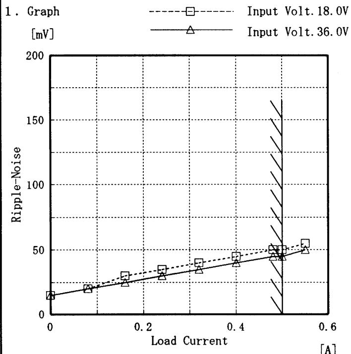
Ripple-Noise is shown as p-p in the figure below.
