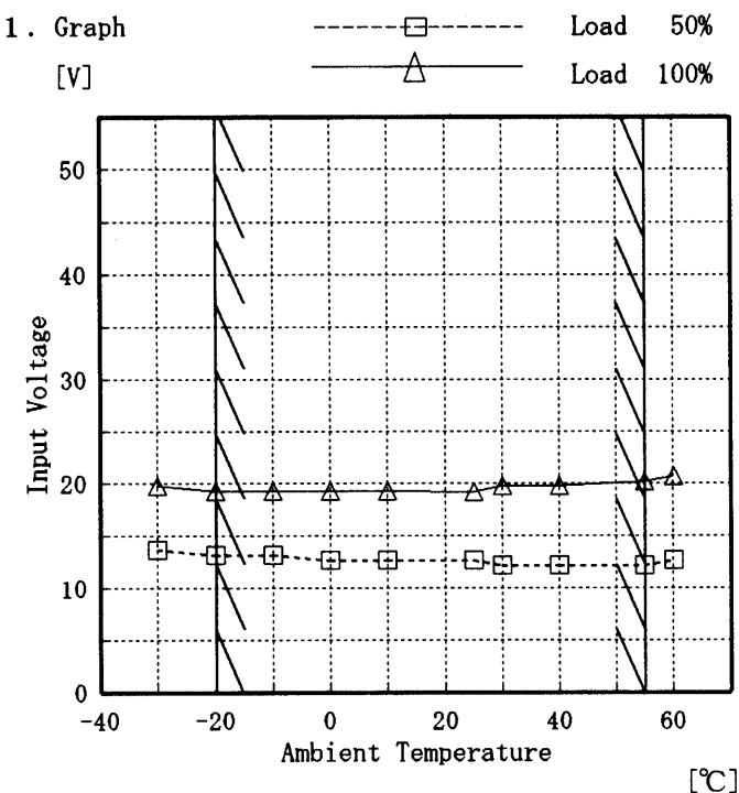
Note: Slanted line shows the range of the rated ambient temperature.
