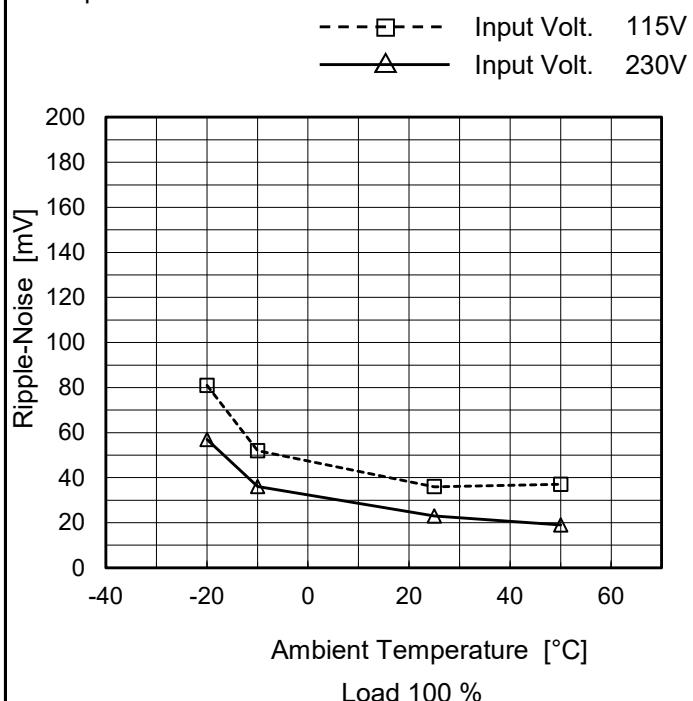
Measured by 20 MHz Oscilloscope.
