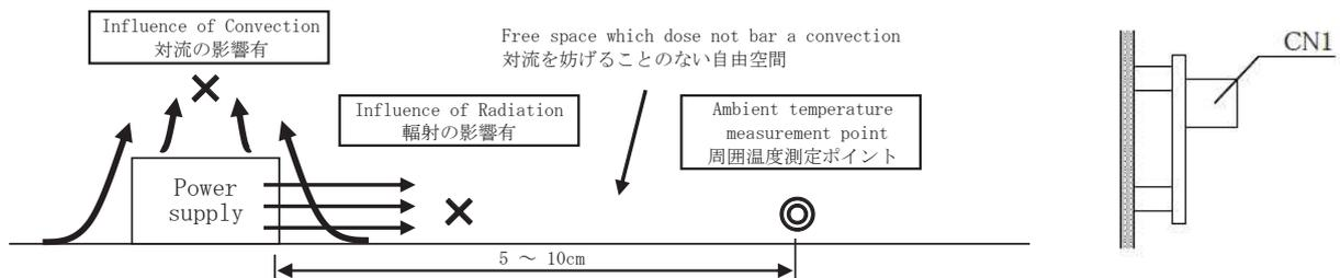
With the ambient temperature of graph, it measures in the environment of a figure.
