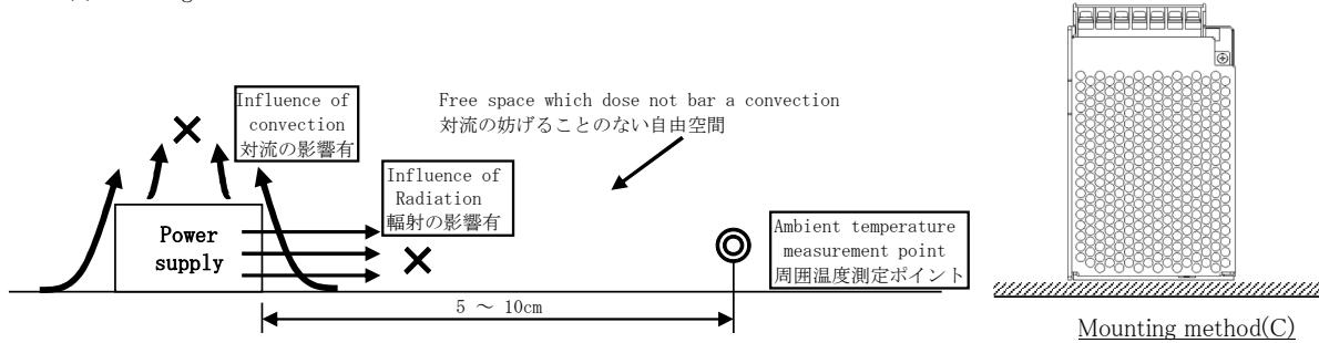
With the ambient temperature of graph, it measures in the environment of a figure.
