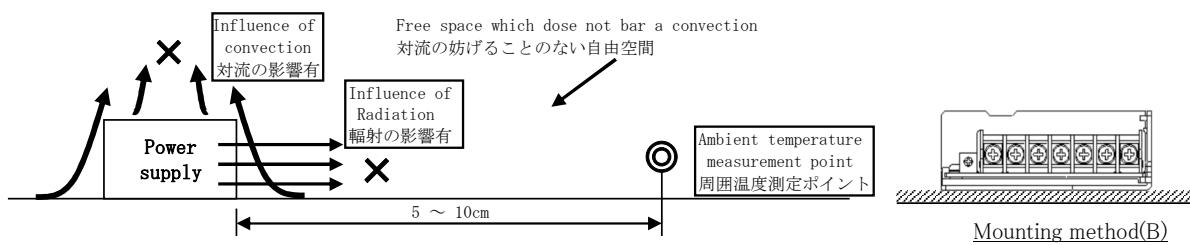
With the ambient temperature of graph, it measures in the environment of a figure.
