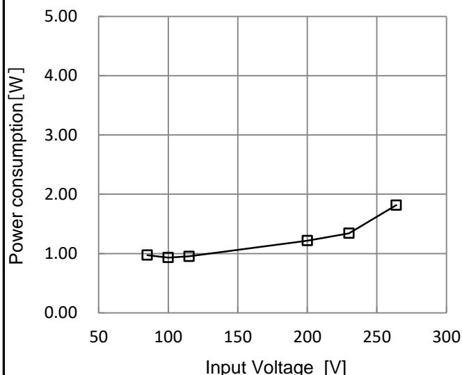
Reducing standby power is possible by OFF signal of the remote control.
