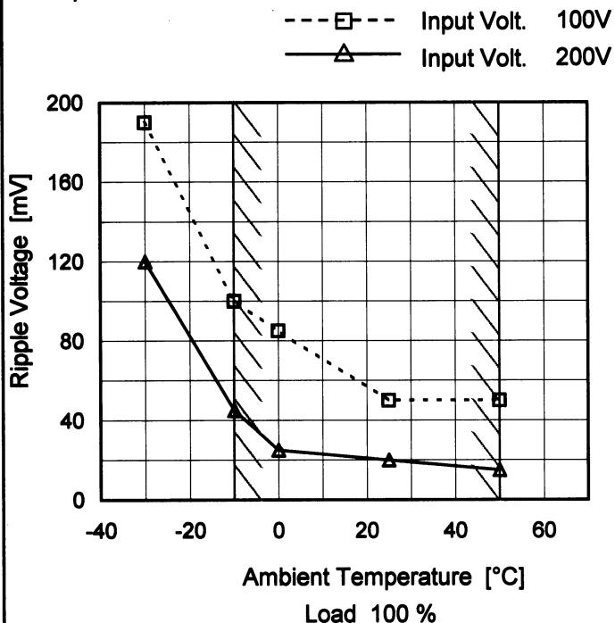
Measured by 20 MHz Oscilloscope.
