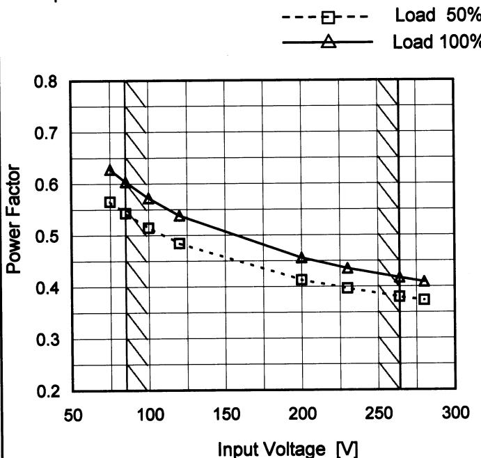
Note: Slanted line shows the range of the rated input voltage.
