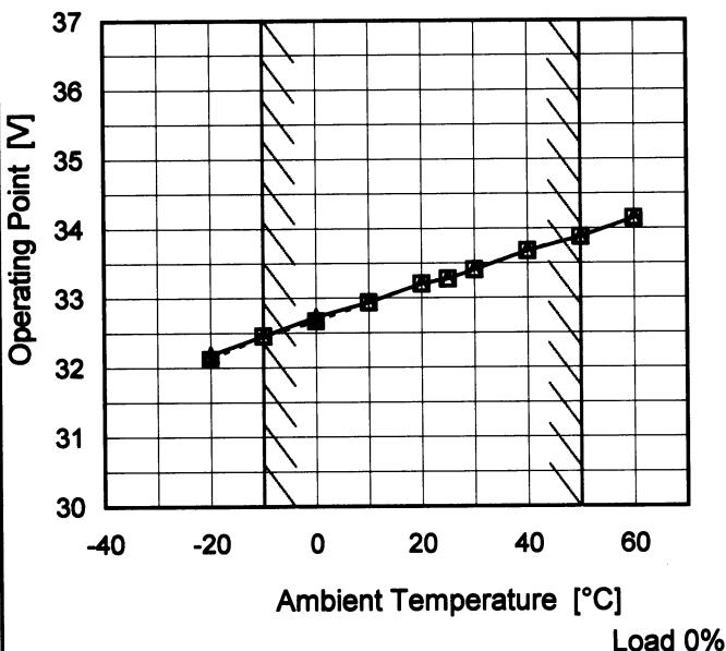
Note: Slanted line shows the range of the rated ambient temperature.
