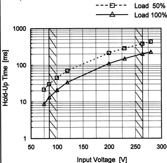
This duration covers from Shut-off of input voltage to the moment when output voltage descends to the rated range of voltage accuracy.
