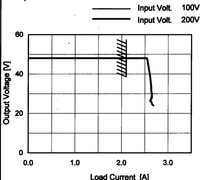
Note: Slanted line shows the range of the rated load current.
