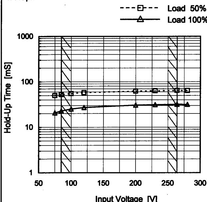
This duration covers from Shut-off of input voltage to the moment when output voltage descends to the rated range of voltage accuracy.
