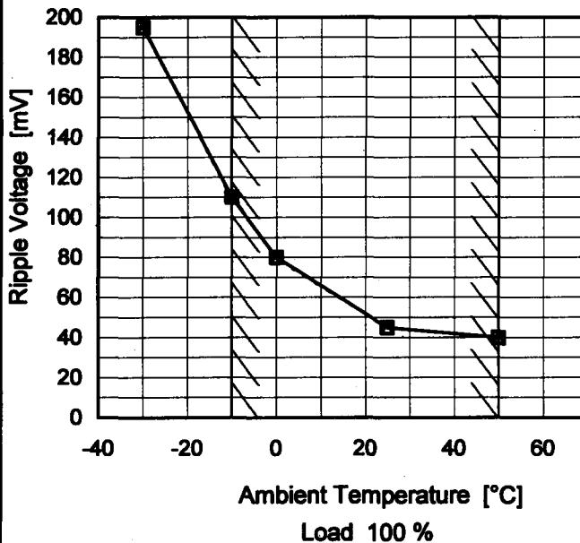
Measured by 20 MHz Oscilloscope.
