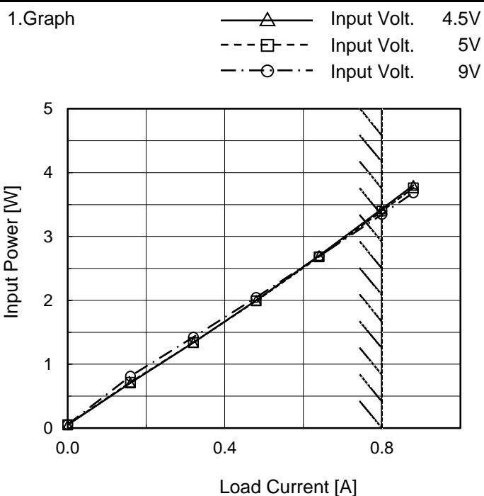
Note: Slanted line shows the range of the rated load current.
