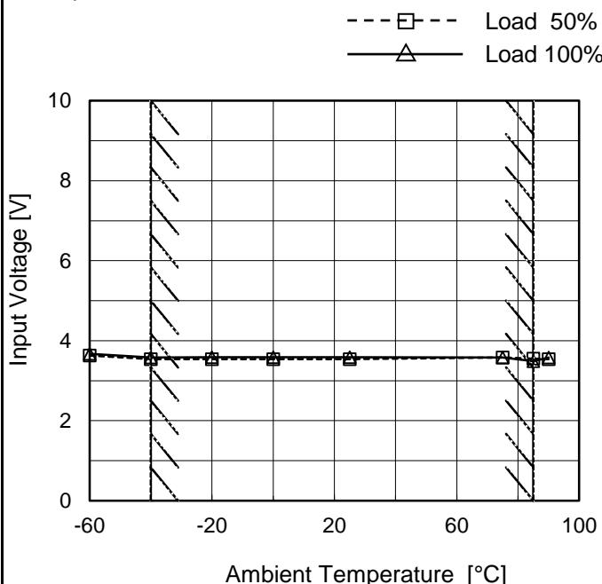
Note: Slanted line shows the range of the rated ambient temperature.
