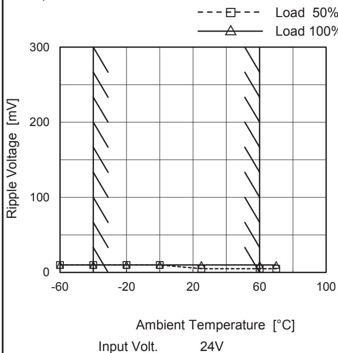
Measured by 100 MHz Oscilloscope.
