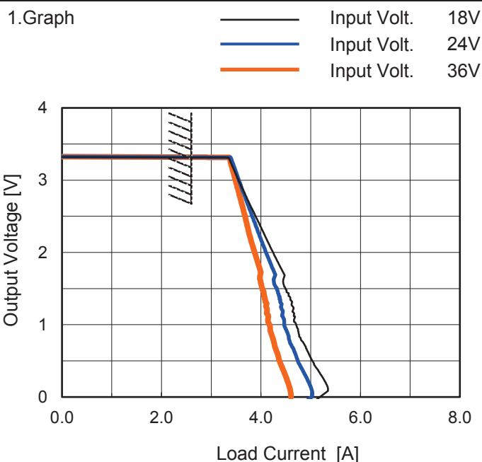
Note: Slanted line shows the range of the rated load current.
