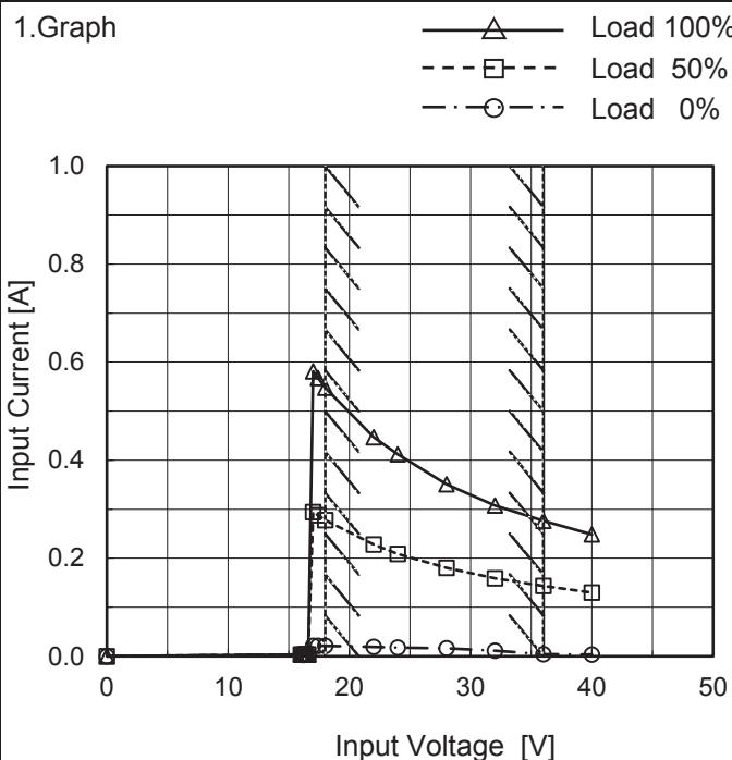
Note: Slanted line shows the range of the rated input voltage.
