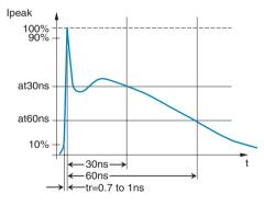
Figure 5.5.1 Discharge current waveform
