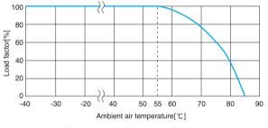
Figure 2.2.1 Derating Curve
