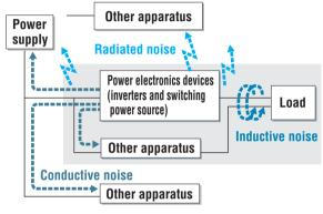
Figure 1.4.1 Propagation Paths of Noise
