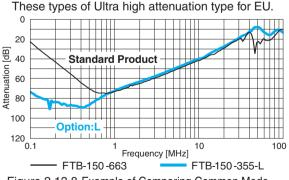
Figure 2.13.8 Example of Comparing Common Mode Attenuation Characteristics between Standard Product and L-option Product
