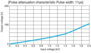
Figure 1.7.3 Example of Pulse Attenuation Characteristic(NAP-16-472)
