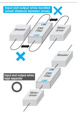
Figure 3.2.2 Input and output wires
