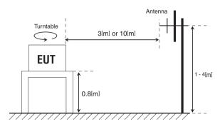
Figure 5.3.1 Example of Radiated Emission Measurement Configuration
