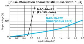
Figure 2.11.2 Example of Comparing Pulse Attenuation Characteristics
