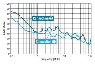
Figure 4.2.2 Example of Effed of Filter Orientation on Noise
