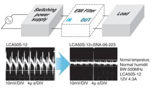
Figure 1.7.2 Example of Effectivemess of Ripple Noise Filter
