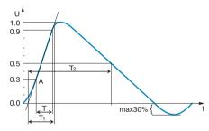
Figure 5.8.1 Example of a Surge Waveform in Voltage
