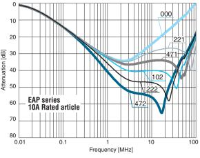
Figure 2.12.1 Example of Ground Capacitor Codes and Common Attenuation Characteristics
