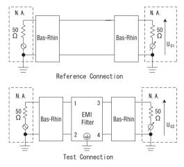
Figure 2.10.1 Attenuation Characteristic Measurement Method (Single-phase Normal Mode)
