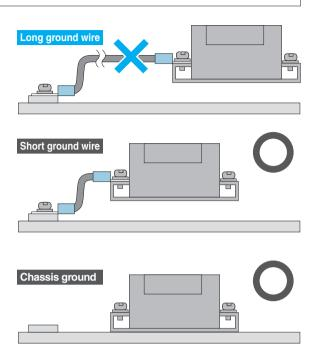
Figure 3.1.2 Proper grounding
