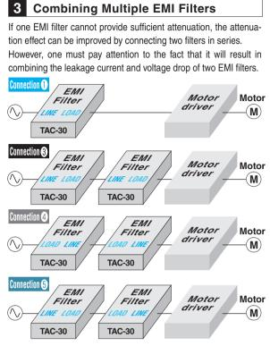
Figure 4.3.1 Example of EMI Filter Connection Directions
