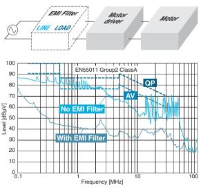
Figure 1.7.1 Example of Noise Reduction by an EMI Filter
