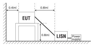
Figure 5.2.1 Example of Conducted Emissions Measurement Configuration
