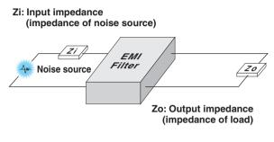
Figure 4.1.1 Input/output Impedances of an EMI Filter Circuit
