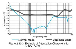
The attenuation characteristic of EMI filters is affected by the input and output impedances of a measured circuit.
