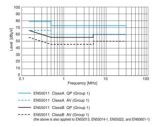
Figure 5.14.1 Conducted Emission Limit Graph
