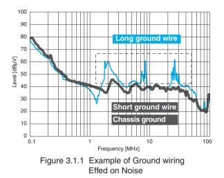
If customers connect the metal chassis of their EMI filter, they can obtain an effect similar to a short ground wire.
