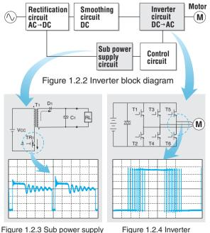
Figure 1.2.3 Sub power supply inverter operation waveform
