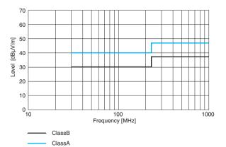
Figure 5.14.2 Radiated Emission Limit Graph
