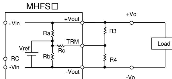
$$V_o = \frac{(1/R_a + 1/R_b + 1/R_c) - (1/R_c)^2 \times (1/R_c + 1/R_3 + 1/R_4)^{-1}}{(1/R_a + 1/R_c) \times (1/R_3) \times (1/R_c + 1/R_3 + 1/R_4)^{-1}} \times V_{ref}$$
