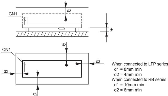
Fig.3.1 Installation method
