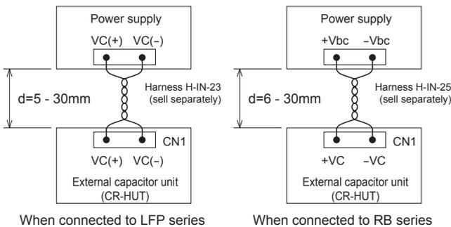
Fig.3.3 Connection method
