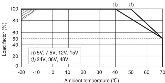
UMA30F-SN Ambient temperature derating curve at rated input
