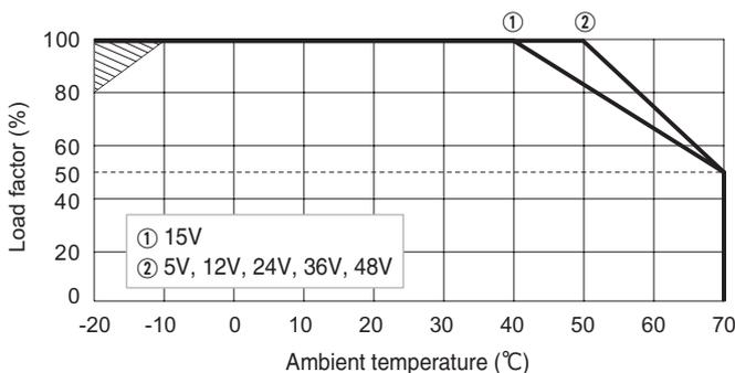
UMA60F Ambient temperature derating curve at rated input
