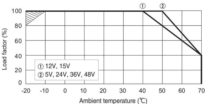
UMA60F-SN Ambient temperature derating curve at rated input
