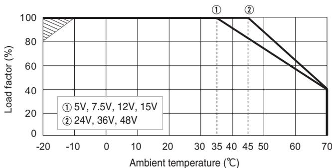
UMA120F Ambient temperature derating curve at rated input
