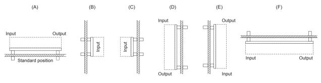
■Option-N model can be mounted in the mounting position shown in the figure below. The installation of (F) possible only forced air cooling.
