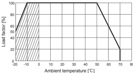
● **PJA600F/1000F/1500F Ambient temperature Derating Curve**
