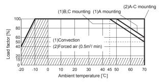
PDA100F Ambient temperature derating curve (Reference value)
