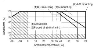
▶ PDA150F-12, -15, -24 Ambient temperature derating curve (Reference value)
