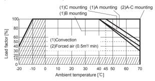
PDA100F-□-N Ambient temperature derating curve (Reference value)
