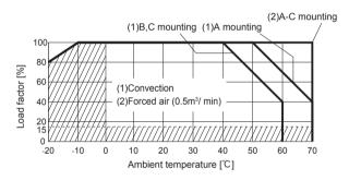
PDA150F-5 Ambient temperature derating curve (Reference value)
