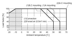
PDA150F-5-N Ambient temperature derating curve (Reference value)
