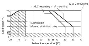
PDA150F-12-N, -15-N, -24-N Ambient temperature derating curve (Reference value)
