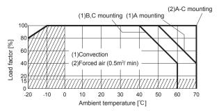
PDA50F-12-N. -24-N Ambient temperature derating curve (Reference value)
