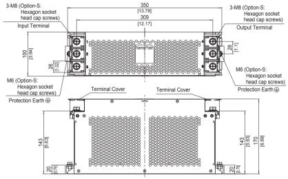
\* The air hole for heat radiation is not on the opposite side side.
