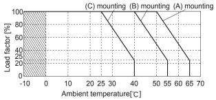
\*In case of ADA1000F-24, load factor 100% means output 24V, 21A at ACIN100V, 24V, 25A at ACIN200V.
