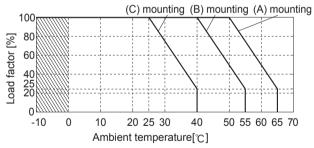
In case of ADA750F-24, load factor 100% means output 24V, 17A at ACIN100V, 24V, 19A at ACIN200V.
