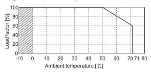
\*In case of ADA600F-24, load factor 100% means output 24V, 21A at ACIN100V, 24V, 25A at ACIN200V.
