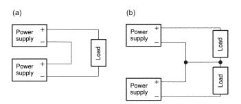
■As variance of output current drew from each power supply is maximum 10%, the total output current must not exceed the value determined by the following equation.
