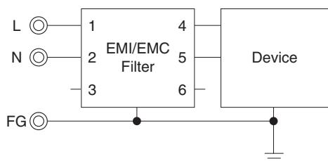
※Three-phase three-wire EMI/EMC filter is also available as a Single-phase input type.
