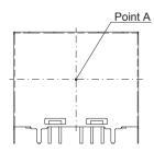
Fig. 7.9 Temperature Measuring Point in the case of Forced Air Cooling
