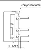
Fig.10.1 Clearance to user board
