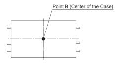
Fig. 7.8 Temperature Measuring Point in the case of Forced Air Cooling (Upper Surface of the Case)
