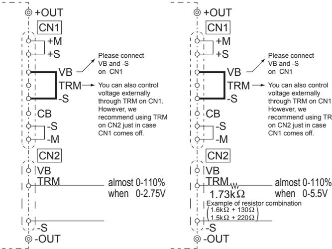
Fig.1.1 Wiring 1
