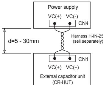
Fig. 7.14 Connection method
