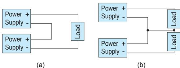
Fig.2.1 Examples of connecting in series operation
