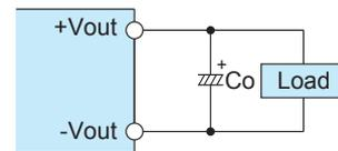
Fig. 7.17 Output side external capacitor connection method
