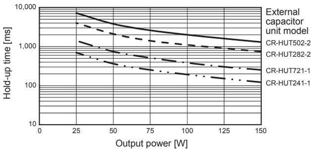
Fig. 7.15 Hold-up time by LHP150F-□-U1Y (Reference data)
