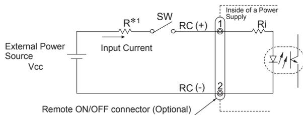
Fig. 7.2 Example of using a remote ON/OFF circuit
