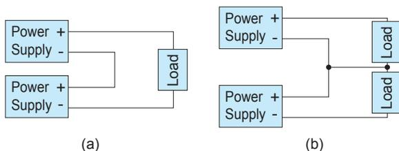
Fig.2.1 Examples of connecting in series operation
