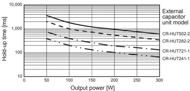
Fig. 7.16 Hold-up time by LHP300F-□-U1Y (Reference data)
