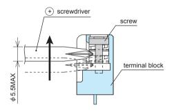
Fig.7.3 lifting method
