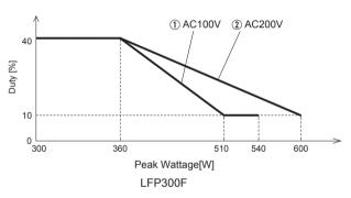
Fig.6.1 Derating of peak loading
