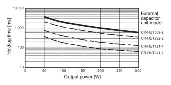
Fig.7.5 Hold-up time by LFP240F- U1Y (Reference data).
