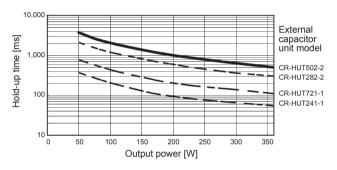
Fig.7.6 Hold-up time by LFP300F
