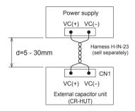
Fig.7.7 Connection method
