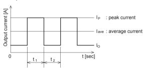
$$t_1 \leq 10 \; [\text{sec}], \; \text{l}_{\text{ave}} = \; \frac{|I_{\text{p}} \; t_{\text{i}} + I_{\text{o}} \; t_{\text{z}}|}{|t_{\text{i}} + t_{\text{z}}|} \leq \text{rated current,}$$
