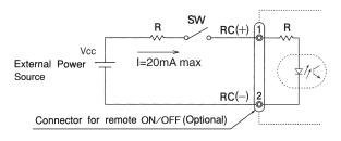
■When external power source is in the range of 4.5 - 12V (LDA300W: 4.5 - 12.5V), current limit resistance R is not required. However, when external power source exceeds 12V (LDA300W: 12.5V), current limit resistance R must be connected.
