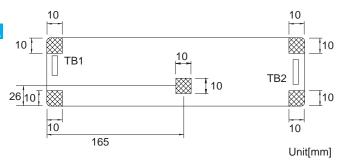
■Keep isolation distance between screw and internal components in case of option "-S", "-SN", as below chart.
