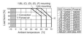
The rated power is different depend on Forced Air/Convection cooling (Please refer Chart in right hand side).
