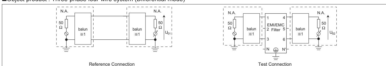
※1 Equilibrium measurement with mixed-mode S-parameters in the instrument
