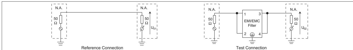
■ Object product : Three-phase three-wire system (Differential mode)
