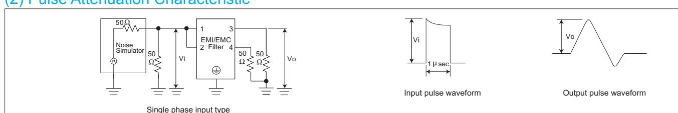
Fig.3.7 Pulse attenuation measurement diagram
