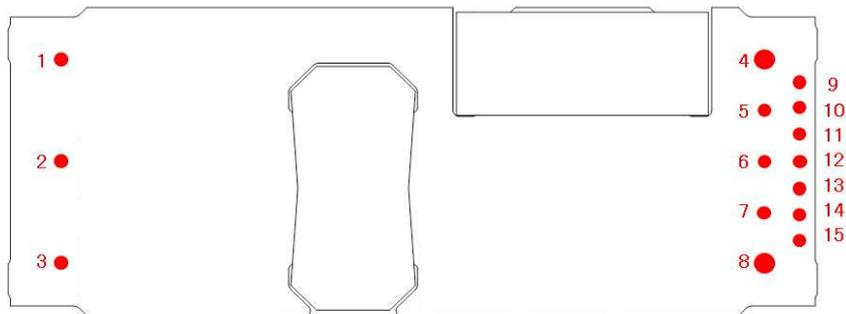
Figure 1-1.1. pin assignment in CHS300-I (top view)
