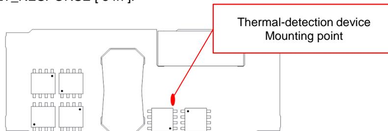
Figure 6-3.1 Temperature measuring point for CHS300-I (top view)
