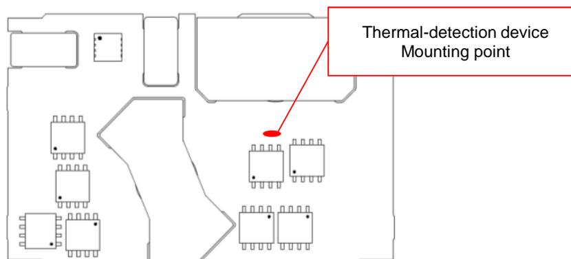
Figure 6-3.2 Temperature measuring point for CHS400-I (top view)
