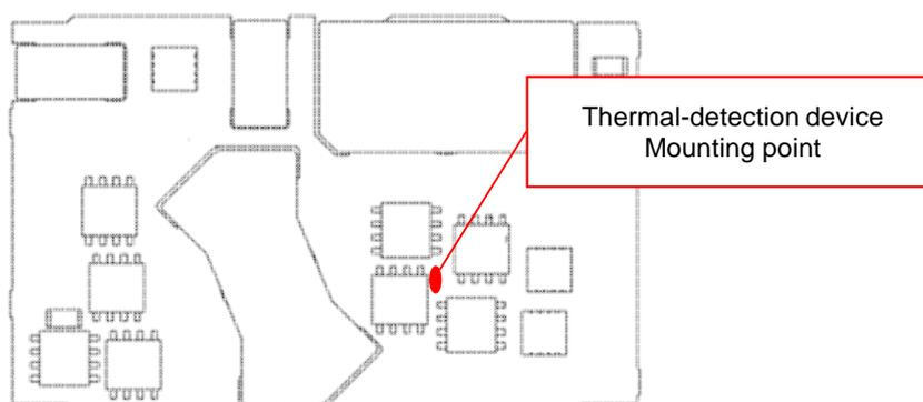
Figure 6-3.3 Temperature measuring point for CHS500-I (top view)
