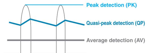
Figure 5.13.1 Relations between Detection Methods and Measurement Levels
