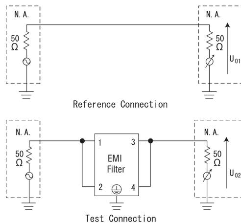
Figure 2.10.2 Attenuation Characteristic Measurement Method (Single-phase Common Mode)
