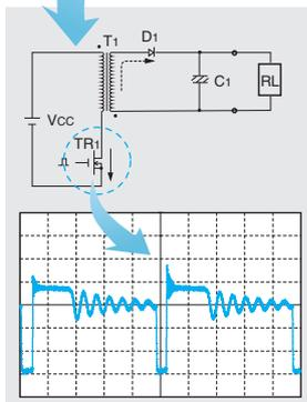
Figure 1.2.3 Sub power supply inverter operation waveform
