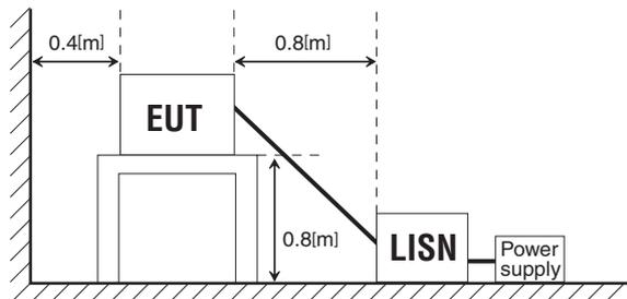
Figure 5.2.1 Example of Conducted Emissions Measurement Configuration
