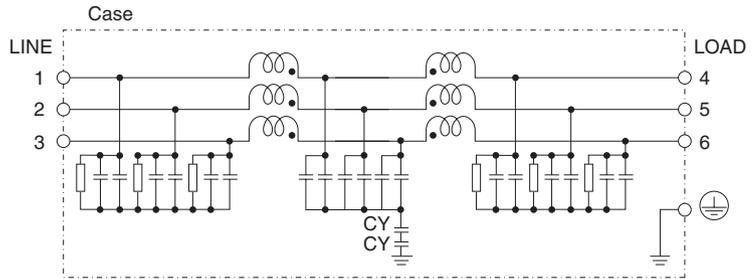
Figure 4.2.4 TBC Series Circuit Diagram (Circuit Is Symmetric)
