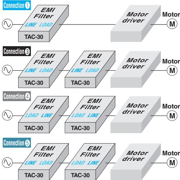
Figure 4.3.1 Example of EMI Filter Connection Directions
