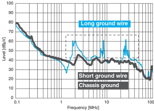
Figure 3.1.1 Example of Ground wiring Effed on Noise
