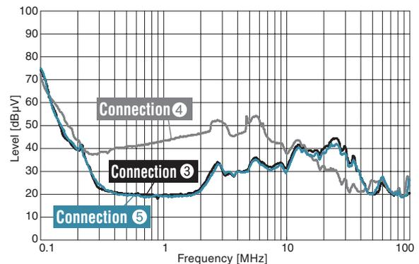
Figure 4.3.4 Comparing Effects of Different 2-filter Configurations
