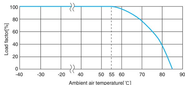
Figure 2.2.1 Derating Curve
