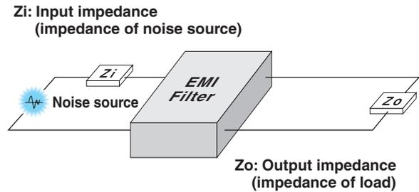
Figure 4.1.1 Input/output Impedances of an EMI Filter Circuit
