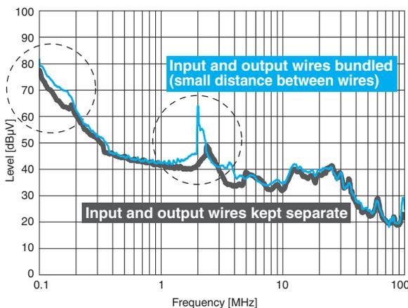
Figure 3.2.1 Example of Effect of wiring on Noise
