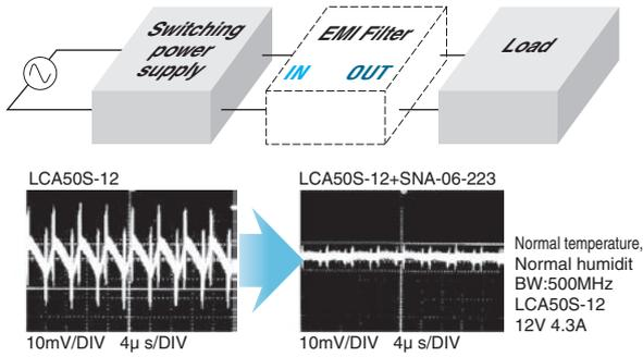
Figure 1.7.2 Example of Effectiveness of Ripple Noise Filter
