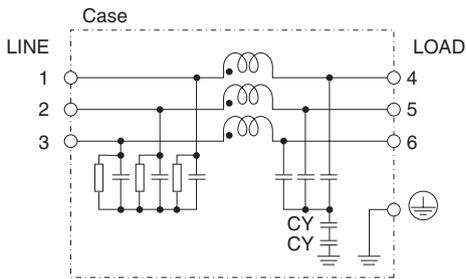
Figure 4.2.3 TAC Series Circuit Diagram (Circuit Is Asymmetric)
