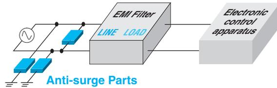
Figure 1.7.4 Proper Installation Location of surge Countermeasures
