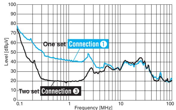
Figure 4.3.2 Example of Effect of Combining Multiple Filters
