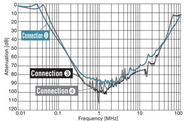
Figure 4.3.3 Comparing Static Characteristics of Different 2-filter configurations
