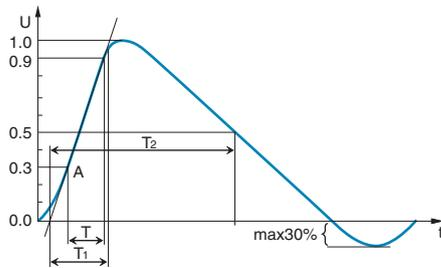
Figure 5.8.1 Example of a Surge Waveform in Voltage
