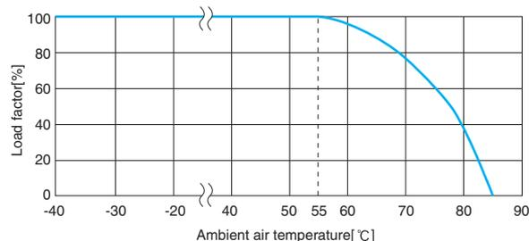
Figure 2.2.1 Derating Curve
