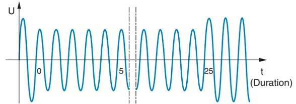
Figure 5.11.1 Example of a Waveform of Voltage Dips
