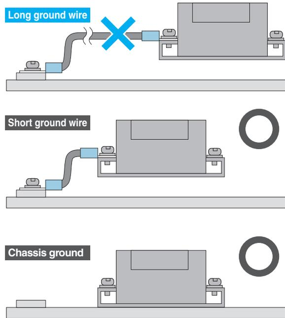
Figure 3.1.2 Proper grounding
