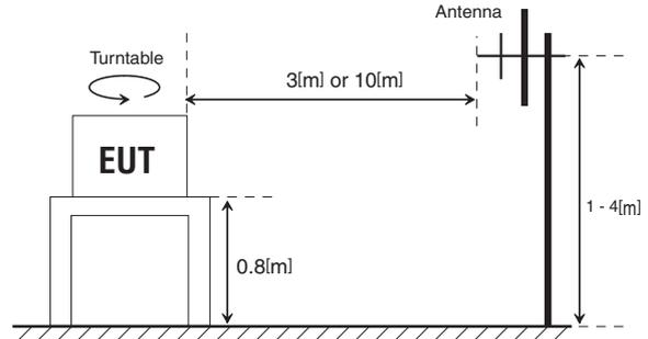
Figure 5.3.1 Example of Radiated Emission Measurement Configuration
