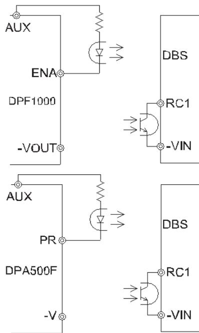
(3) Auxiliary power supply circuit for external signal (AUX)
