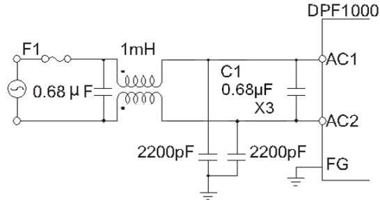
(3) External capacitor on the input side C1
