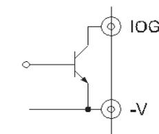
(2) Enable signal (ENA) /Power Ready signal (PR)
