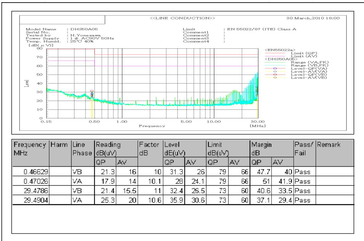
■ Fig. 10.4 shows the recommended circuit of noise-filter which meets CISPR Pub. 22 Class A and the noise level.
