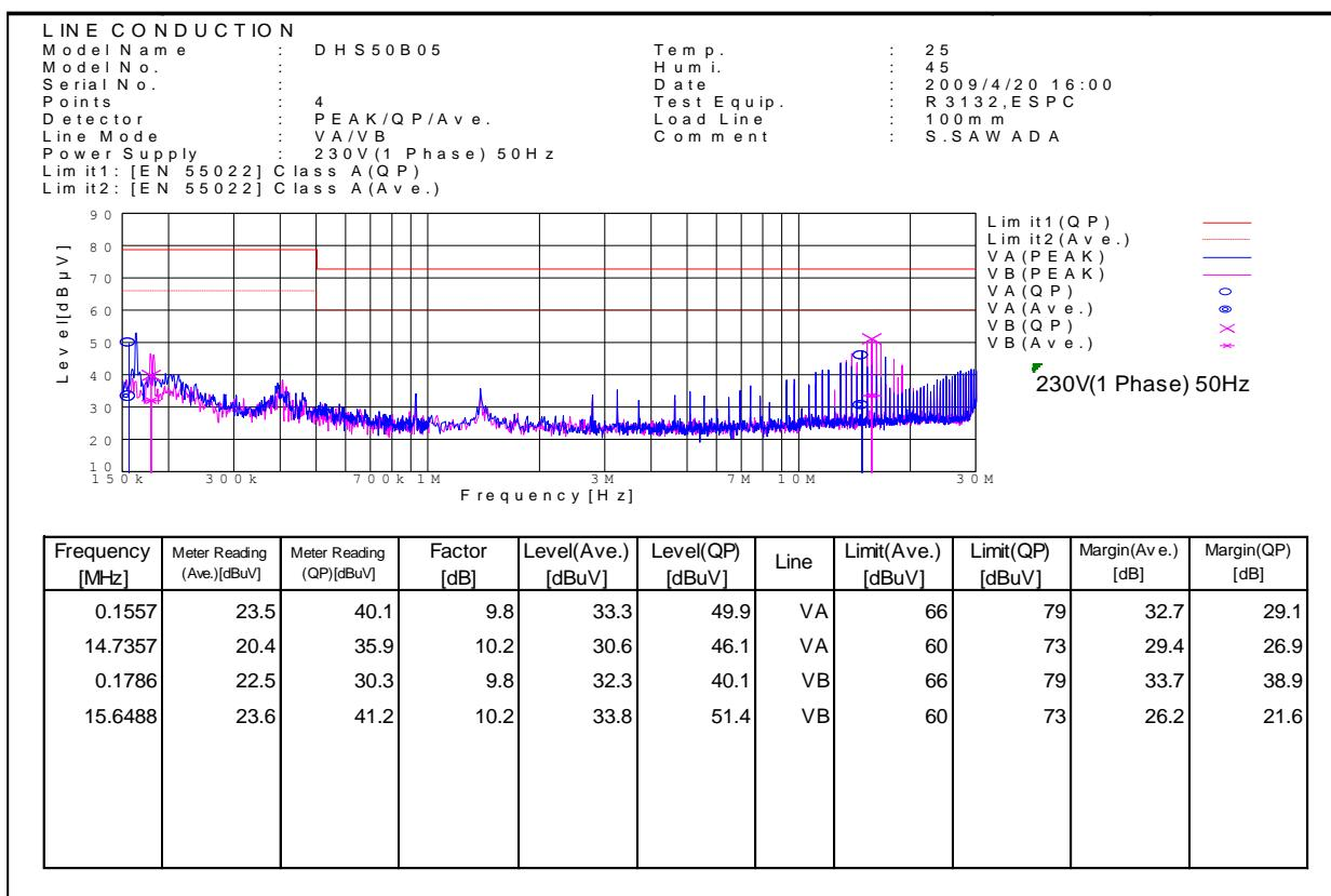
■ Fig. 10.5 shows the recommended circuit of noise-filter which meets CISPR Pub. 22 Class A and the noise level.
