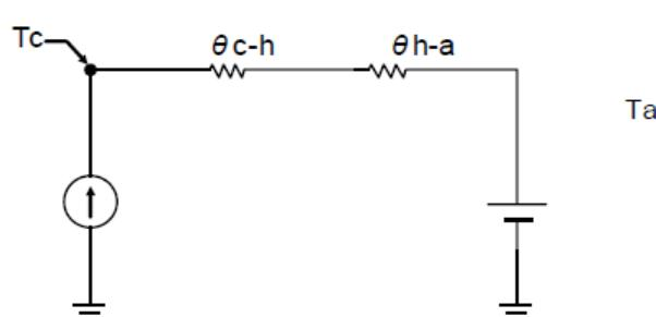
The thermal resistance of heat sink is calculated by following equation.
