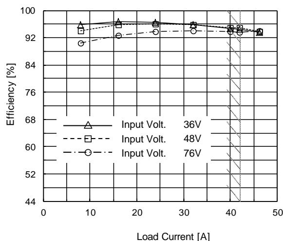
(c) Efficiency ( by Load Current )
