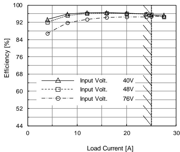
(c) Efficiency ( by Load Current )
