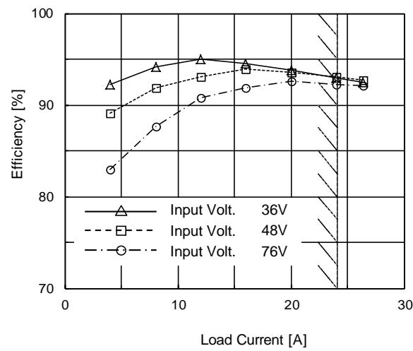
(c) Efficiency (by Load Current)
