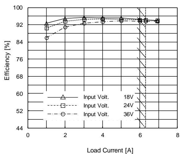
(c) Efficiency ( by Load Current )
