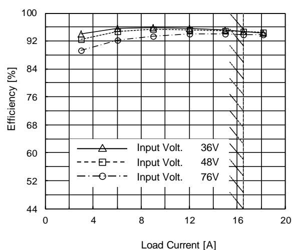
(c) Efficiency ( by Load Current )
