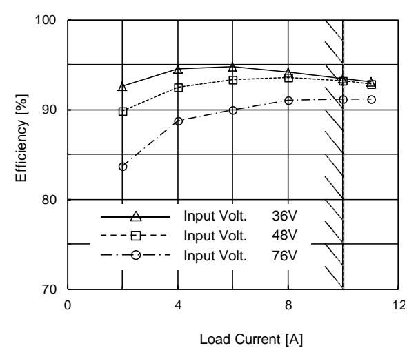
(c) Efficiency ( by Load Current )
