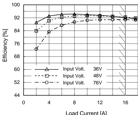
(c) Efficiency ( by Load Current )
