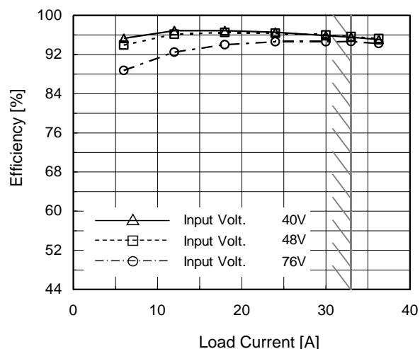
(c) Efficiency ( by Load Current )
