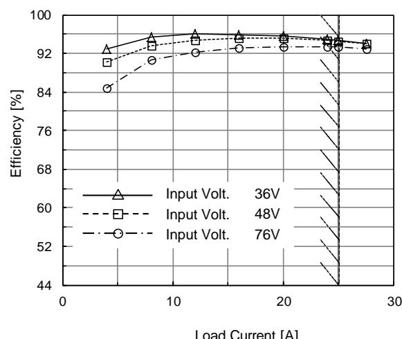
(c) Efficiency ( by Load Current )
