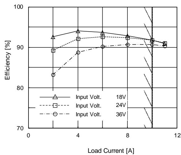
(c) Efficiency ( by Load Current )
