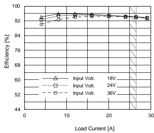
(c) Efficiency ( by Load Current )
