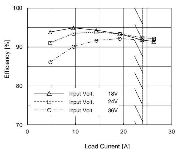
(c) Efficiency ( by Load Current )
