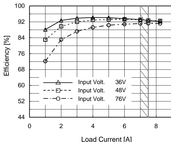
(c) Efficiency ( by Load Current )
