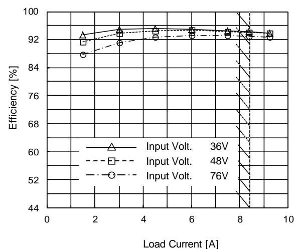
(c) Efficiency ( by Load Current )
