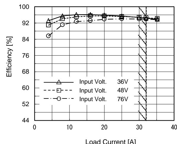
(c) Efficiency ( by Load Current )
