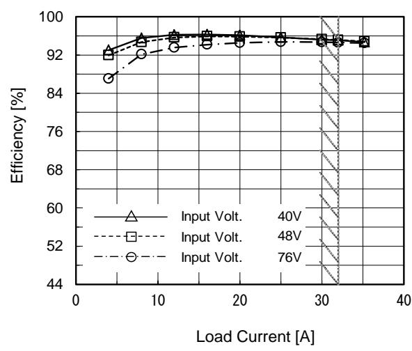
(c) Efficiency ( by Load Current )
