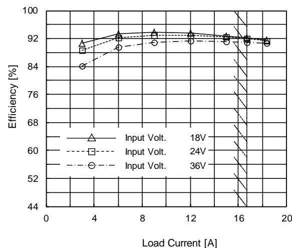
(c) Efficiency ( by Load Current )
