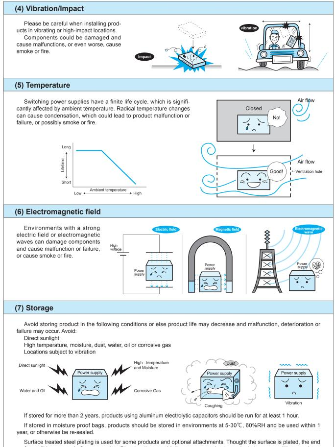
Surface treated steel plating is used for some products and optional attachments. Thought the surface is plated, the end surface will be exposed after processing. Discoloration or oxidation may occur due to product storage conditions or placement, but this will not affect product performance or reliability. If this is a concern and protection of the end surface is required, please contact us.
