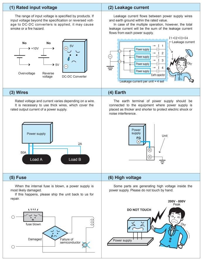
Generally, switch mode power supplies are designed to operate in controlled environments (e.g. inside the office). The products should have a special care because some operating conditions may cause a malfunction or failure of the products, smoke or fire at the worst case.
